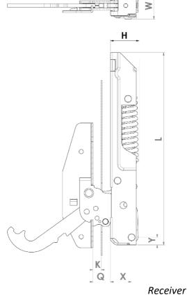
Hole fixation spacing: 85mm Side fixation available
